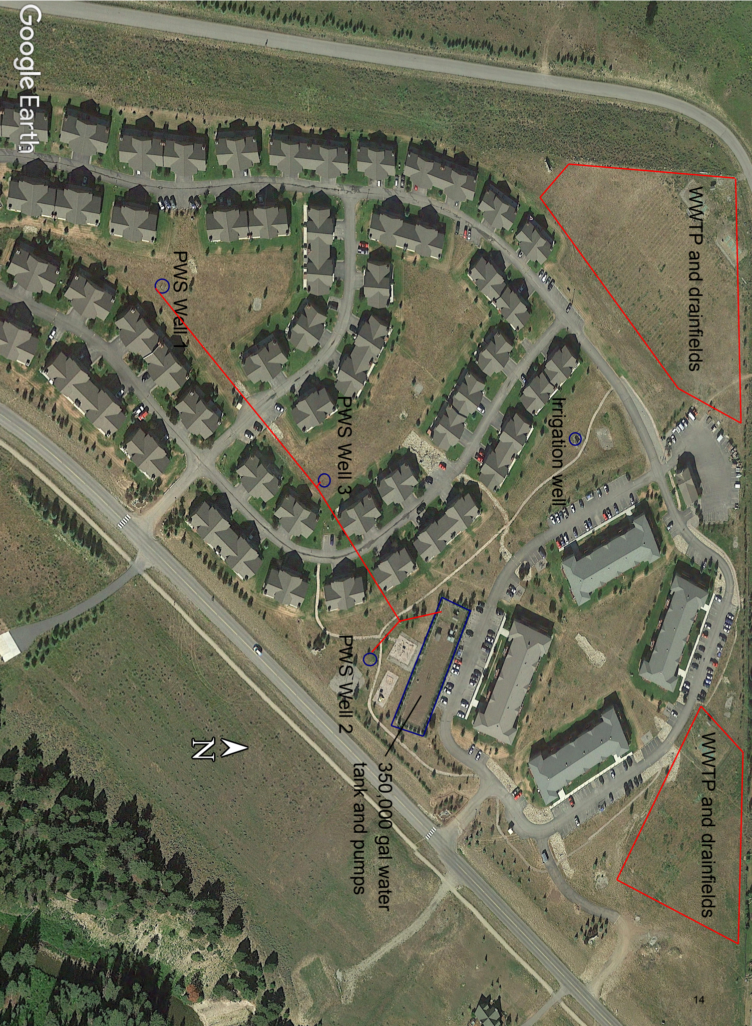
Approx. locations of major water/wastewater system components
